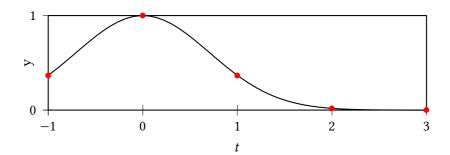
The plot contains the analytical solution and the five output points of the numerical solution as red dots. They lie exactly on the analytic solution.
